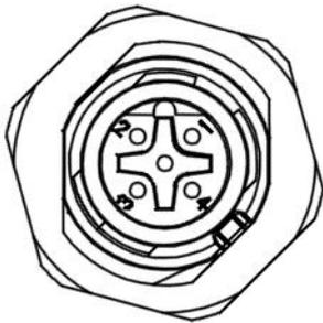
Figure 1: View of the X2b connection
