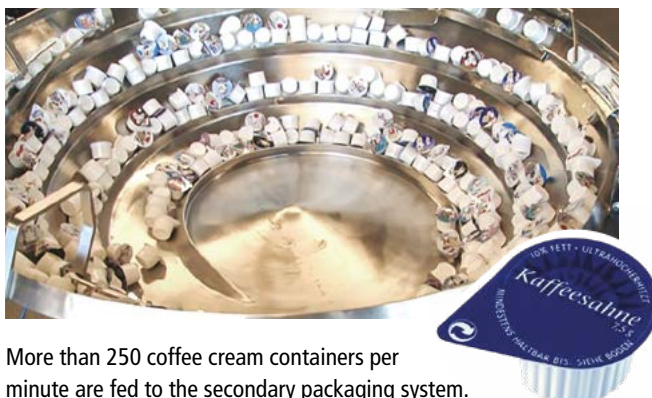
Flexible feeding components such as the aflex enable the separation of parts of different geometries and are suitable for versatile applications due to short changeover times.
