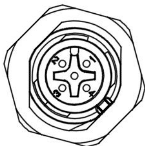
Figure 10: Vue des branchements [X2a]
